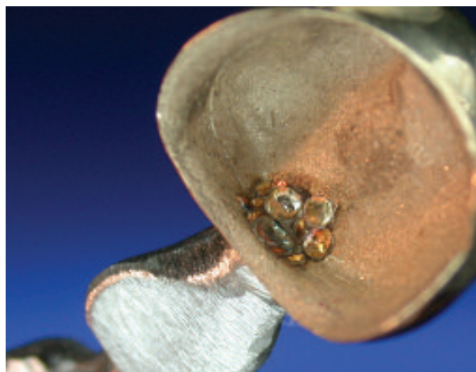
Fig. 28: Since the welding spots are in general concave, it is not necessary to refit the crown to the die after welding
