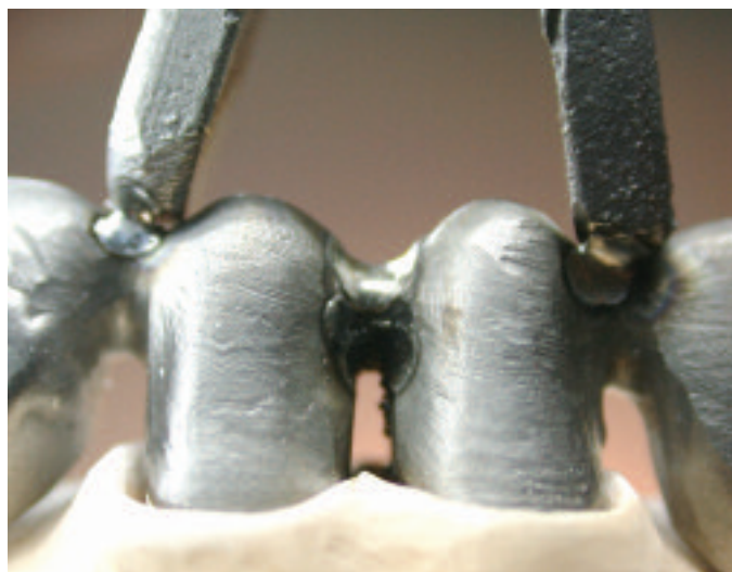
Fig. 11: "Classic" interproximal cut, edges beveled, then phaser welded as described, with perfect passive fit
