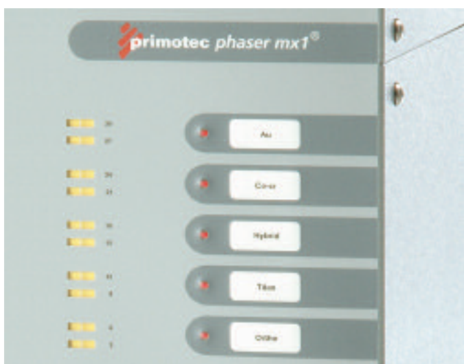
Fig. 14: Primotec phaser mx1 preset programs for Gold, Cobalt-Chrome, Hybrid (Gold to Co-Cr), Titanium and orthodontics
