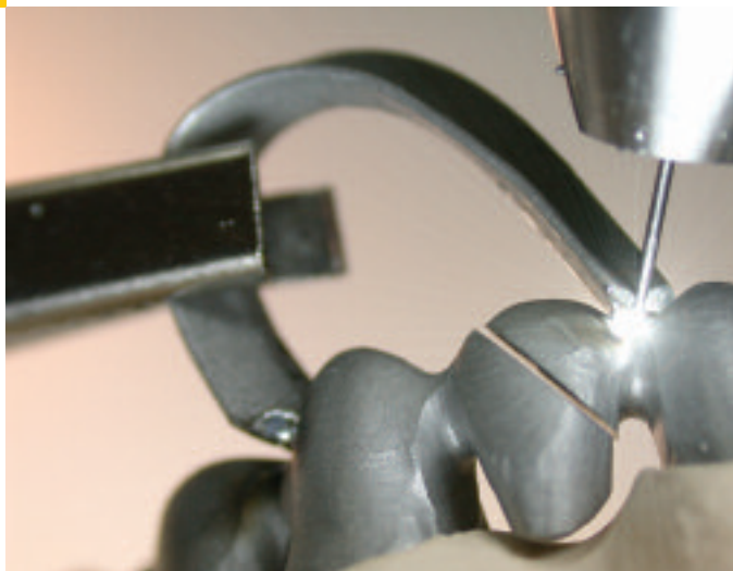
Fig 15: Diagonal cut through the pontic. The wide gap requires filling with welding wire. The bent bar welded on top secures the position and prevents distortion.
