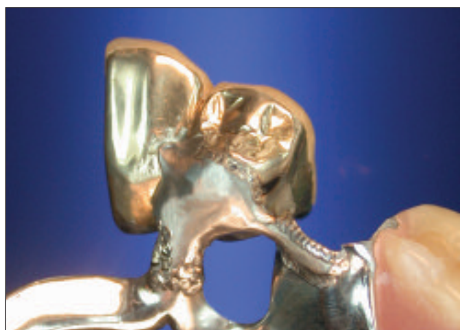
Fig. 5. The secondary crowns had broken off. They were welded back to the CoCr-partial without removing the pink acrylic or the veneers
