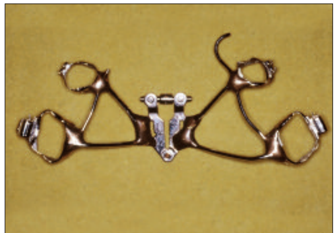
Fig. 2. Corrosion on orthodontic appliances can show different discolorations depending on the solders used.
