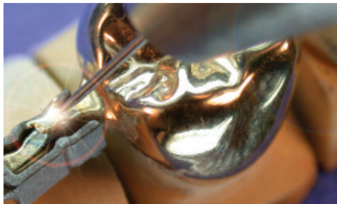
Fig. 9: Telescopic secondary gold crown joined to Co-Cr partial. In this case the first fixing impulses are done without wire.
