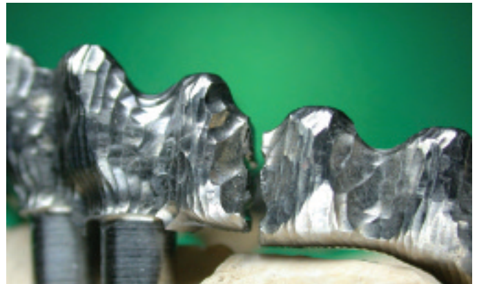
Fig. 30: Before drilling the holes, the two pieces must be screwed to the model with the same defined torque that will be used later on in the patient's mouth.
