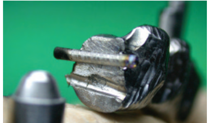
Fig. 32 and 33: one wire is welded to the lower groove of the one piece; the other wire-pin is welded to the upper groove of the other piece.
