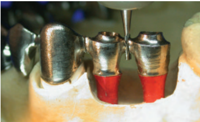
Fig. 19: next, a parallel round bur of the same size as the wire to be inserted is used.
