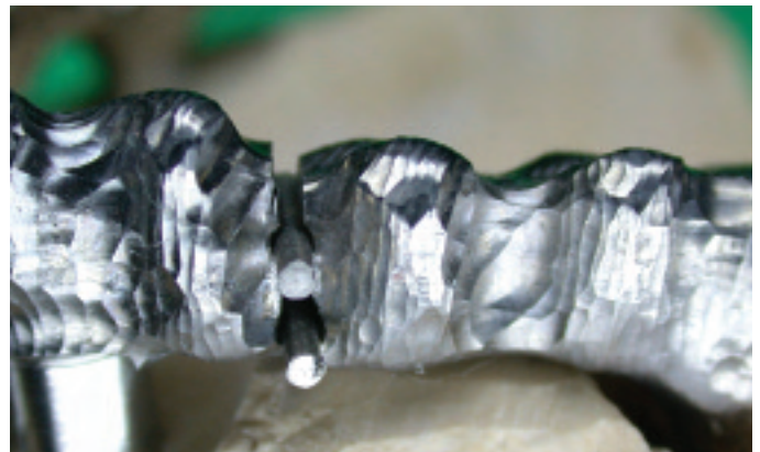
Fig. 31: the two wire pins in place. Since the gap was larger in width than in height the holes to house the wire pins had been drilled horizontally.
