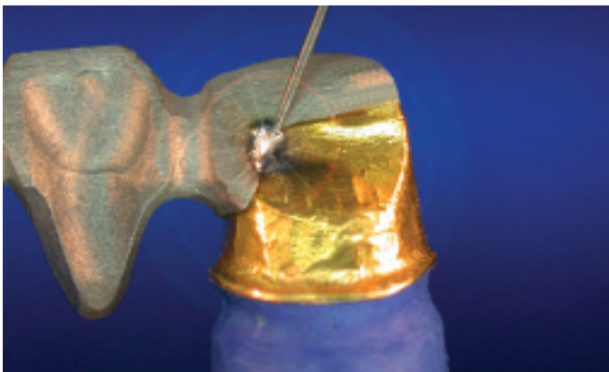
Fig. 13: always aim at the cast alloy, never at the coping or the gap in between. It may take some impulses on the same spot before the cast alloy will melt the gold and both fuse together.
