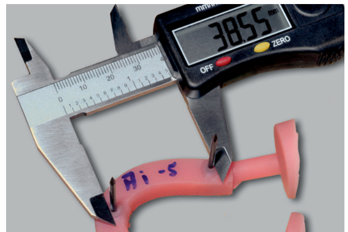
Figs 10 and 11 The same measurements are taken of the test pieces reproduced in acrylic as on the original, in other words the distances at the tips of the pins and at the point where the pins enter the acrylic. These values are then compared with those of the original.
