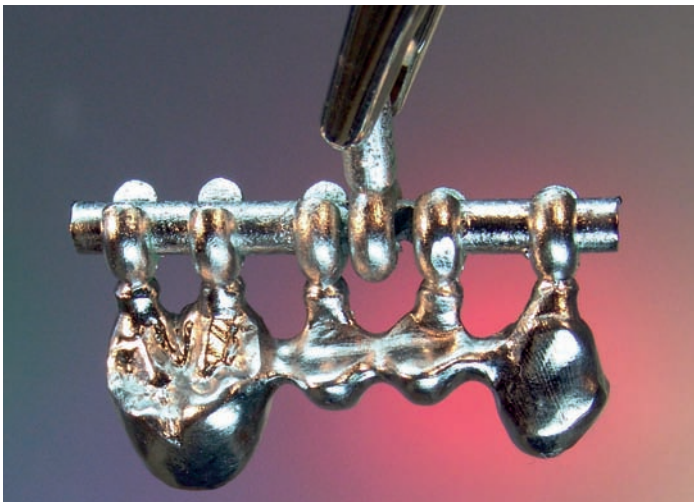
Fig. 21: A perfect casting result obtained with less alloy
