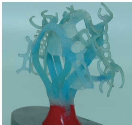
Fig. 6: The mobile magnetic cone is used to move the wax-ups to their optimal position on the muffle base
