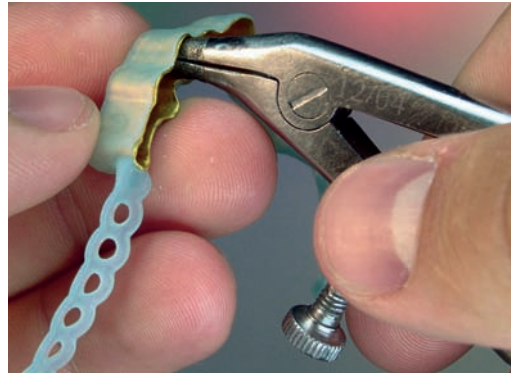
Fig. 36: The pink wax between the electroplated coping and the tertiary framework is heated through the gold layer by hot telescope pliers. The electroplated copings will drop out of the polymerized wax-up.
