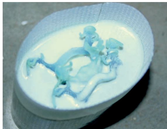
Fig. 8b: Vertical investing reduces the risk of bubble formation on the castings
