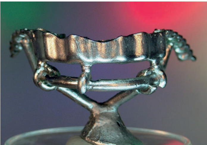
Fig. 39: Speed-cast, divested and sandblasted tertiary structure
