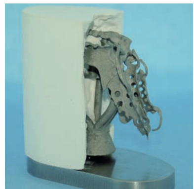
Fig. 7: A clean triple casting, only half divested for demonstration purposes. It is apparent how much investment compound can be saved, and only one casting reservoir was used.
