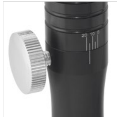
Arto 3 Bennett angle adjustable from 0° to 20°
