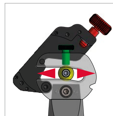
Condyle fully opened, condyle sphere moves freely, centric screw is deactivated.
