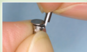
Bend the locking key and brake it.
