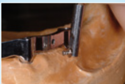
Create a hole in the wall of the bar using a 1.6 mm ball drill.
