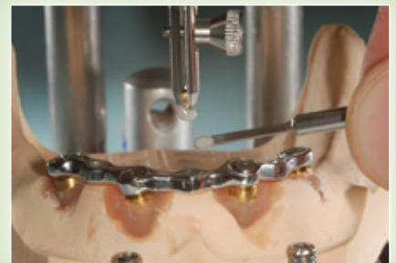
Place the assembled attachment into the parallelometer key. Use a self curing metal to metal bonding composite on the sleeve and in the cylinder.
