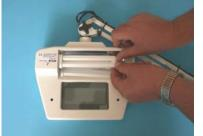
32. Unpack all parts and check to make sure that everything is complete. Install the light bulb in the socket on the underside of the magnifying glass.
