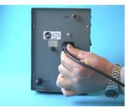
7. Plug the power cord into the power receptacle (socket). Attention: Do not plug the power plug into the power outlet until you have completed installation.
