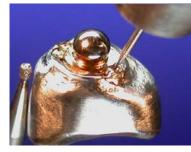
1. In this example, Bona-type ball attachments are to be welded as retention elements to root canal posts made of a nonprecious alloy.
