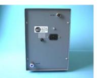
6. View of rear panel with power receptacle (socket), fuse holder, argon gas connection and plug sleeve for the shutter.
