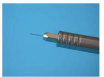
44. Close the clamping chuck, tightening by hand. Do not use a wrench.
