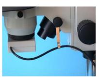
26. ... carefully screw it on (without damaging the threads) and hang the shutter cord on the designated hook.
