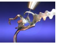
7. In this case, you do not need to use any additional welding wire for the basal side. Don't forget that Co-Cr has to be welded slowly.
