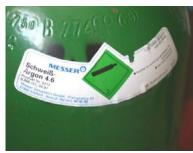
60. Finally, you have to connect the primotec Phaser mx1 control unit to a gas tank containing argon 4.5 (this equals a purity of 99,995%)
