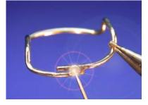
2. ... elements overlap a bit. After the first joining impulse, weld the seam so that the weld spots always overlap by 50%.
