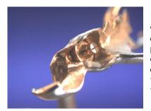
1. To be able to weld an HSL anchor onto the cast partial, you must expose it on the occlusal side. With the workpiece on the model,...
