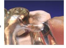
6. Next, select the hybrid program and weld the joining element to the secondary crowns.
