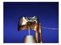
3. Now you can weld additional welding material spot-by-spot onto the proximal surface.
