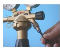
65. Insert the free end of the argon gas hose already connected to the control unit into the quick-connect valve of the pressure regulator.
