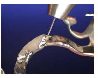
7. ... is still more efficient than having to remove the saddles. After the actual welding is complete, increase the impulse duration and ...
