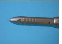
45. The electrode should extend 7-10mm past the handpiece nozzle. Both ends of the electrode can be used before regrinding is necessary.
