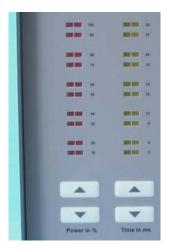
Use the "Power" and "Time" (impulse duration) keys to change these welding parameter individually.
