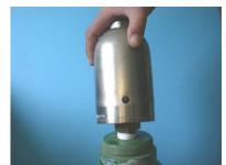
63. First, the gas bottle must be secured so that it cannot fall over. Always comply with current regulations. Then screw off the protective valve cap.
