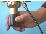
68. You can regulate the gas flow rate with the valve on the bottom of the pressure regulator. Set four liters per minute (reading is shown on the right gauge).
