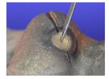
3. Always place your first joining impulse at the site where the gap between the two bridge elements is smallest.
