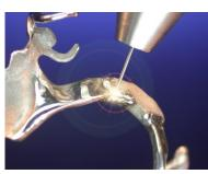
6. ... but weld massive seams "from the inside out". This work is tedious and will take several minutes, but compared to soldering, ...
