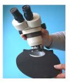
21. Insert the microscope into the ring of the microscope holder
