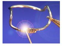
3. Five to six impulses should be sufficient to achieve a solid, permanent seam. Then you can easily use rotary instruments...
