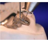
2. Join the retention with a few spot welds, and then weld the seam (if necessary, reduce the gas preflow time to save argon).
