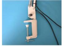
34. Insert the swivel arm of the magnifying glass down into the corresponding hole of the vice clamp. The arm should now swivel freely to either side.
