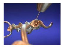
2. ... place the first spot welds. Then you can remove the workpiece from the model and finish welding.
