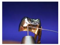
1. To achieve a spherical contact, start applying the material at the equatorial level towards buccalproximal. Be sure to hold the welding wire ...
