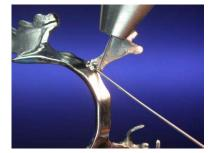
4. Then, weld the retention from the basal. If you are working with welding material, always aim the electrode tip at the welding wire.
