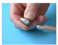
41. The primotec Phaser mx1 comes equipped with 10 special tungsten electrodes, each of them having a service life of at least 1500 impulses.
