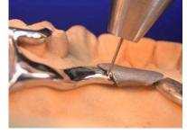
3. ... between the bar halves and the joining element, the less welding material you need. Always complete the weld on one side first, ...
