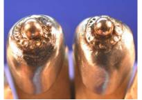
4. Now that you have finished welding on the Bona-type ball attachments, you only have to rubber-wheel and polish the seam weld.
