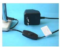
30. The microscope lighting unit has a separate on/off switch on its power cord. This allows you to use the microscope alone, without the primotec Phaser
