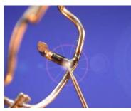
6. Even if you are welding "from the inside", touch the electrode to the ascending occlusal bar to melt the edge on perfectly.
