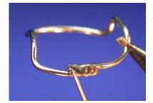
4. ... to finish, rubberwheel and polish. If necessary, of course, you can also counterweld on the inside.
