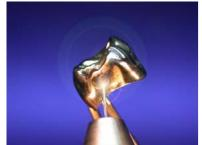
4. For finishing, you can also use the Phaser mx1 to smoothen the spot weld (see page 21), adjust the contact and polish to a finish.
