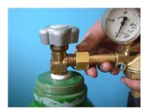
64. Install the pressure regulator as described in the enclosed "Operating Instructions for Cylinder Pressure Control Valves".
