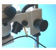
59. Turn the knob on the microscope holder to bring the workpiece into focus. If you cannot achieve a sharp focus, adjust the
