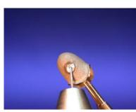
4. In case the wall of the crown in the surrounding area of the hole is too thin, weld on a thin sheet of the same alloy over a wider area.
