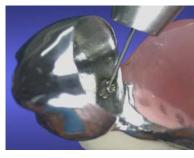
4. If necessary, you can simply weld several layers of welding material over each other.
