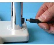
29. Plug the cord of the lighting unit power supply into the designated socket on the bottom rear side of the post.
