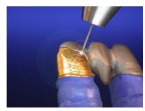
3. Always send your first tacking impulse to the area where the gap between coping and bridge element is the smallest.
