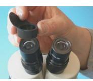
27. Place the rubber eve-cups on the microscope oculars, in such way that the higher side ...
