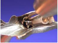
2. Place your first spot weld at the site where you have the smallest distance between attachment and cast partial. Check the fit...
