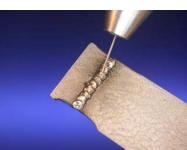
5. ... between the individual impulses. This kind of work should always be welded also from the basal. Since you will usually require welding wire, ...
