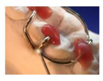
5. If you want to join thick and thin wires together, connect the alligator clip to the thicker wire.
