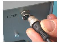
36. Connect the LCD shutter by plugging the cable connecting plug into the female socket labeled "Filter" on the rear panel of the control unit and tighten it securely by hand.
