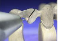
2. In these cases, you can place a hollow seam weld without worrying about the statics. Aim the first welding impulse at the site where the gap ...
