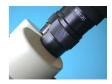
55. The silver line on each eyepiece represents the zero position for the diopter setting.
