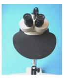
22. ... and, at the same time, attach the light shield between microscope and ring of the holder.
