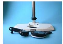
11. Start assembling the parts of the microscope. First, mount the stand for the handpiece to the microscope stand.
