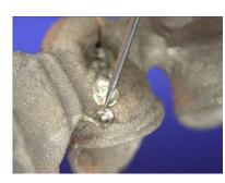
4. Once you have reliably secured the bridge with the first impulses, you can lift the workpiece off the model and weld a circular seam, ...
