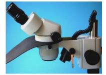
24. The microscope is correctly mounted on the microscope holder.
