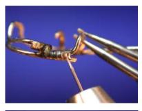
7. Finish all seams to be welded as described above. As with smoothening, you can also weld over the welded areas again, if necessary.
