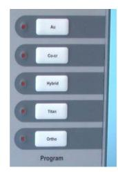
Your Phaser mx1 is factory equipped with five standard programs. To activate one of these programs, simply press the key labeled with the program you would like to run.
