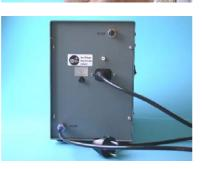
9. Plug the argon gas hose (supplied with the gas connection set) into the quick-connect plug.
