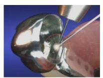
2. Aim the electrode tip at the welding wire and wait until the pulse is triggered.
