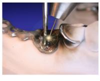
3. To prevent cracks from forming at the weld spots, it is advisable to anneal the Wiptam wire before welding it on.
