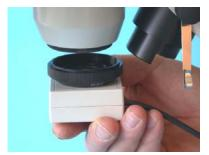
25. ...first unscrew the black protective ring to expose the threads. Bring the shutter into position, ...
