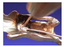
4. Use welding wire to fill any gaps between attachment and cast partial. Always aim the electrode tip at the wire.
