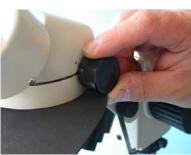
58. The magnification factor can be set infinitely from 1–4 by turning the knobs on both sides of the microscope. This corresponds to a 4–20x magnification.
