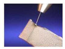
3. With the first spot welds, join the two partial frameworks parts together.
