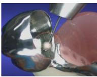
5. To smoothen the welded-on welding material, turn up the impulse duration and reduce the power input accordingly.
