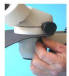
23. Secure the microscope by tightening the fastening screws located on the microscope ring.
