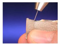
2. ... the new cast extension to fit the existing transversal belt. Allow no gap at all or only a small gap between the parts to be welded.
