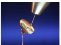
3. ... new margin, you may have to start working with welding material right away. Place several spot welds 360° around the margin to join it securely. Then...
