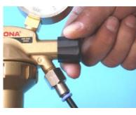
67. Open the valve on the right side of the pressure regulator.
