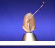
2. Place the welding wire approx. 0.5mm inside the defect. Aim the electrode tip exactly at the welding wire.
