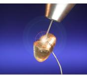
6. Pulse-by-pulse a 360° weld is created. **As a rule of thumb:** Where the parts to be welded parts touch each other, it is possible...
