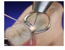
5. As with a modeling instrument, you can now apply material "spot-byspot" with the electrode tip and welding wire.
