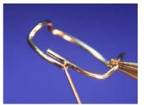
1. In general, you should never butt weld the wire elements end-toend. Instead use short seams so that the bent ...
