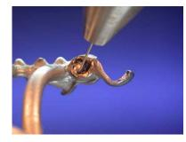
3.Always make sure to weld criss-cross (tighten the wheel nuts) to prevent distortion ...
