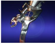
6. ... then weld the basal side. Ideally, the separating gap was as wide as the wire, i.e. you were able to fit the wire into the gap.
