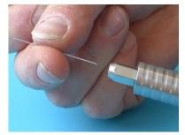
43. Loosen the clamping chuck and insert an electrode into the collet chuck.
