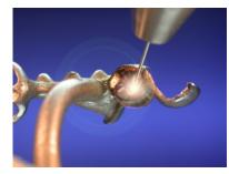
4. ... and use the proper welding material if the gap is still too large. Remember to always aim the electrode tip at the welding wire.
